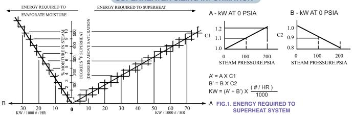
Figure 1 graphically shows the power required to superheat 1000 lbs of steam per hour. The total power required is the sum of the energy required to vaporize the moisture content plus the energy to superheat the vapor. Use Figure 1 to determine the required KW.
